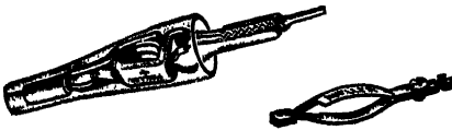
Crocodile clip with rubber insulating sleeve, and a small, plain spring clip for temporary connections.
